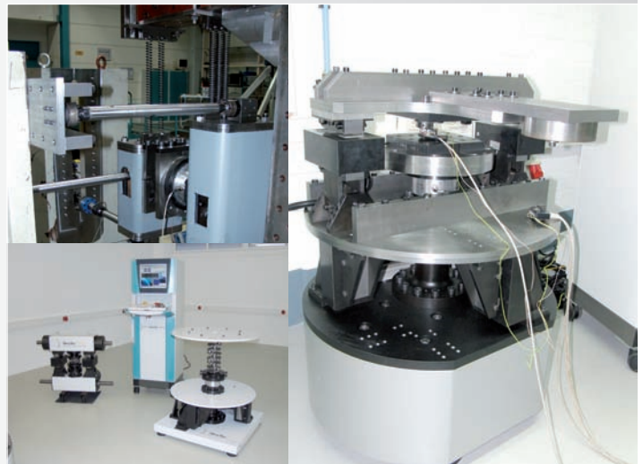
top left: uniaxial resonance test systems below: biaxial hydraulic test system right: biaxial resonance test system
